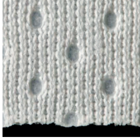
Series 410 ★ double layer knitted polyester wipe with sealed edges, typical surface structure
