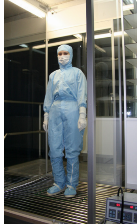
Fig. 3: Test person in cleanroom coverall and suitable accessories during the standing simulation in the Body-Box
