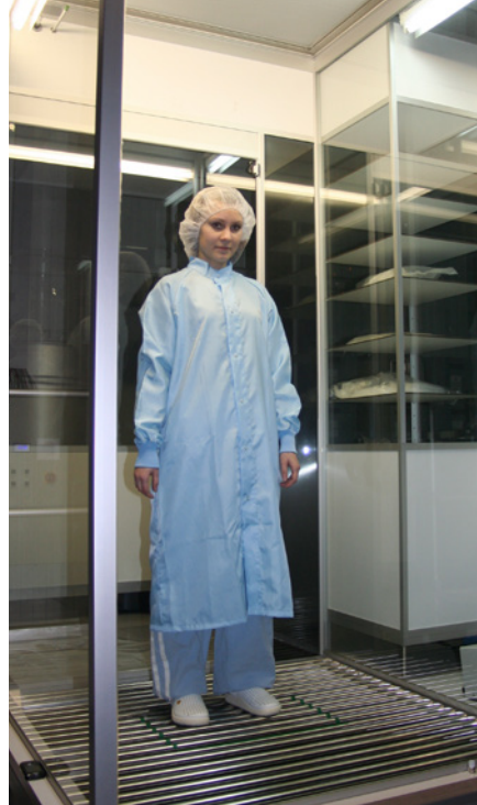
Fig.2: Test person in cleanroom lab coat and suitable accessories during the standing simulation in the Body-Box
